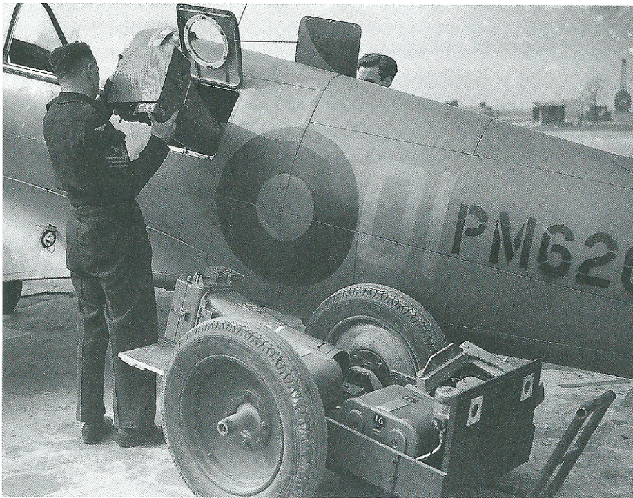
Left: Ground crewman loading an F.52 camera with a 36-in lens into the cramped rear fuselage of a Spitfire PR 19. The film magazine, sitting on the trolley, was attached to the top of the camera after the latter was in place.
