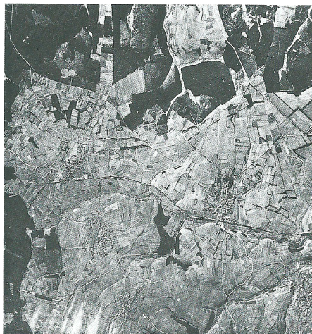
Above: Scale mattered. The village at Bullingen in Belgium (centre right of the picture, nearly halfway up), photographed by 'Shorty' Longbottom during his initial mission on 18 November 1939. Taken from 33,000 feet using an F.24 camera with a 5-in lens, the scale is about 1:79,000. Little ground detail is visible and individual vehicles or troop positions could not be picked out.
